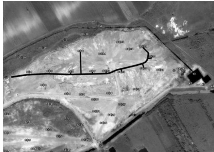
Figure 3: Connected gas extraction wells and main pipeline
