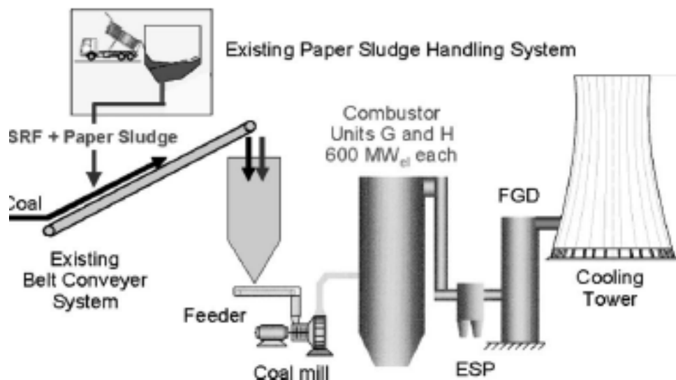
Figure 1: The dosing system for coal, SRF and paper sludge into the steam boiler [5]
